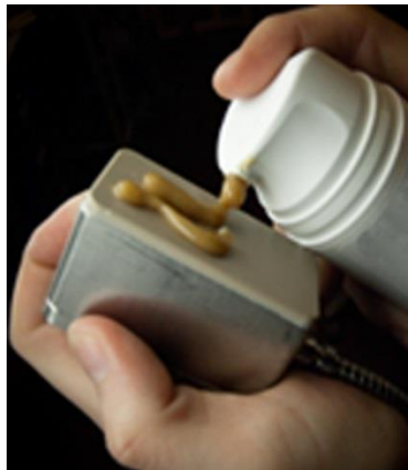
Illustration 5: Application of acoustic coupling gel
